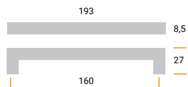
MZA2105 Materiale / Material: Metal Largh. / Width: 8,5 mm. Lungh. / Length 193 mm. Alt. / Height 27 mm. Interasse / Cd 160 mm.
