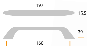
MZ1885 Materiale / Material: Metal Largh. / Width: 15,5 mm. Lungh. / Length 197 mm. Alt. / Height 39 mm. Interasse / Cd 160 mm.
