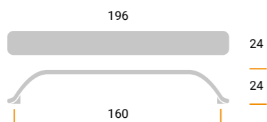
MZA2135 Materiale / Material: Metal Largh. / Width: 24 mm. Lungh. / Length 196 mm. Alt. / Height 24 mm. Interasse / Cd 160 mm.
